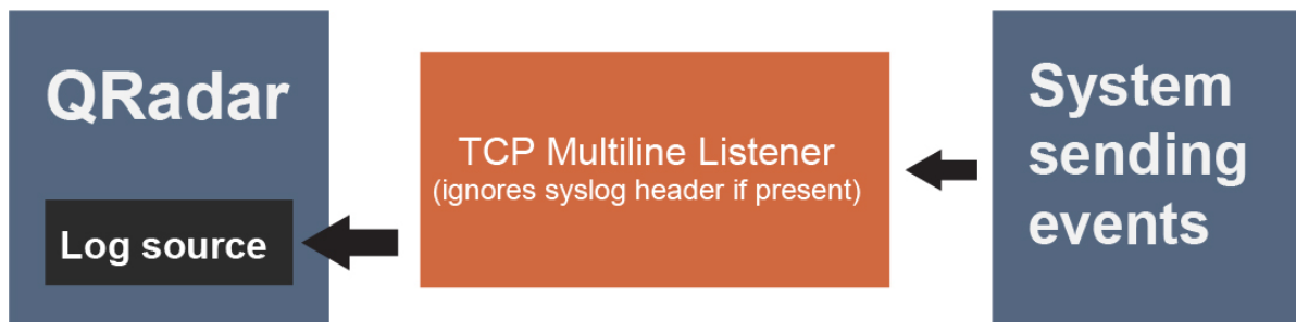
Figure 2. A QRadar log source collects events sent from a single system to a TCP Multiline Syslog Listener
